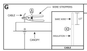
**3:** Use the #16 gauge hole of the AWG wire strippers to strip 1/2" of the outer plastic insulation from the cables.
