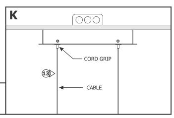
**13:** To make any adjustments to the fixture height, push the cord grips to slide the fixture up and down until the desired height is achieved. Release the cord grips to lock the cables in place.
