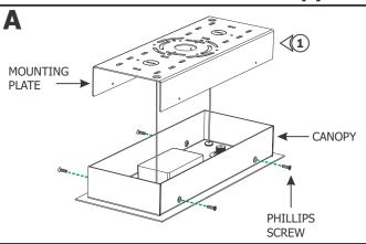
2: Select the appropriate knockout on the mounting plate and remove it using a flathead screwdriver or other appropriate
