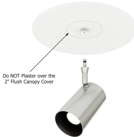
V2P-FJ12 Vanishing Point 2" Flush Canopy to dry wall plaster in and paint, with ELV power supply in J-Box
