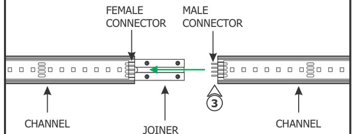
**3:** Lift a section of the lens at the end of the channels where the connectors are visible. Slide the channel over the joiner and ensure the male & female connectors mate properly.
