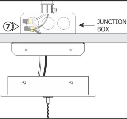
**7:** Place all line voltage wires and wire nut connections inside the junction box.
