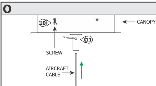
**10:** Align the support canopy holes and secure the canopy in place by tightening the four screws.
