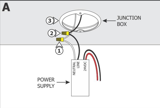
**NOTE:** Before beginning any electrical work, ensure that power to the junction box is turned off.
