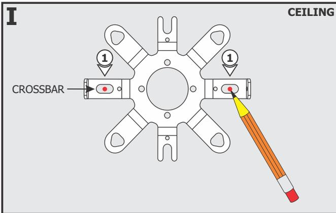
**NOTE:** 4" Support Canopy shown. Omit steps 1 through 5 if using 5" or 6" Surface Mount Support Canopy.
