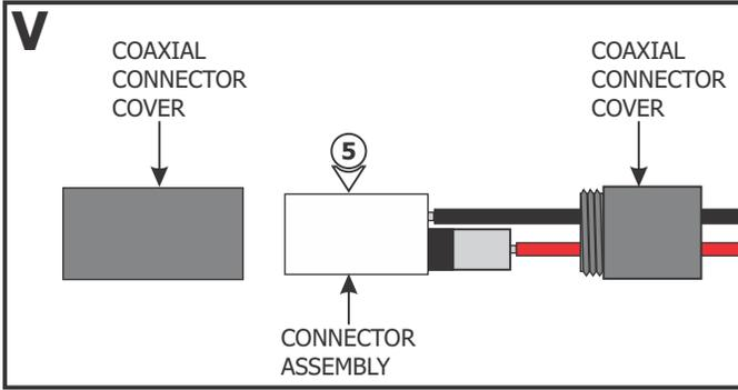
**5:** Unscrew the coaxial connector covers and remove from the connector assembly.
