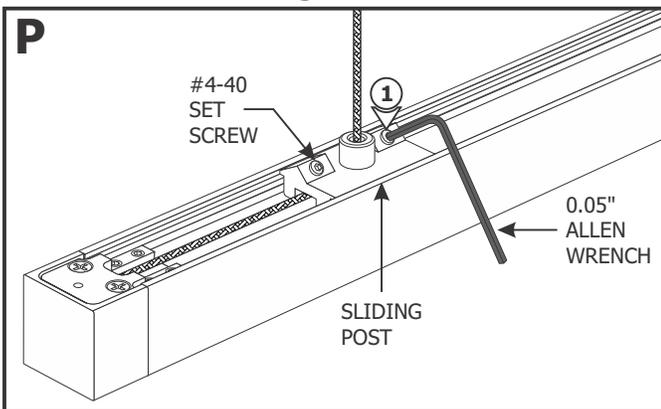
**1:** Loosen (**DO NOT REMOVE**) the two #4-40 set screws on the sliding post with a 0.05" Allen wrench.
