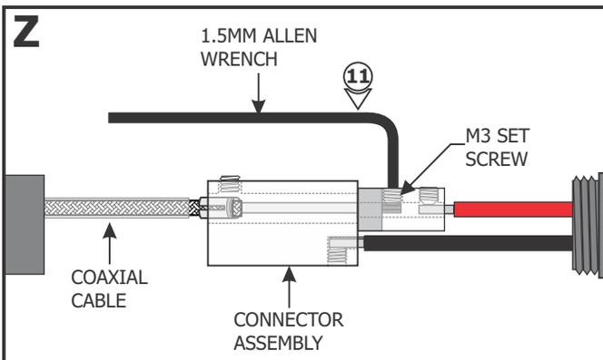
**11:** Use the provided 1.5mm Allen wrench to replace and securely tighten the M3 set screw.
