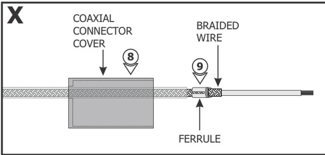
**8:** Slide the connector cover over the coaxial cable.
