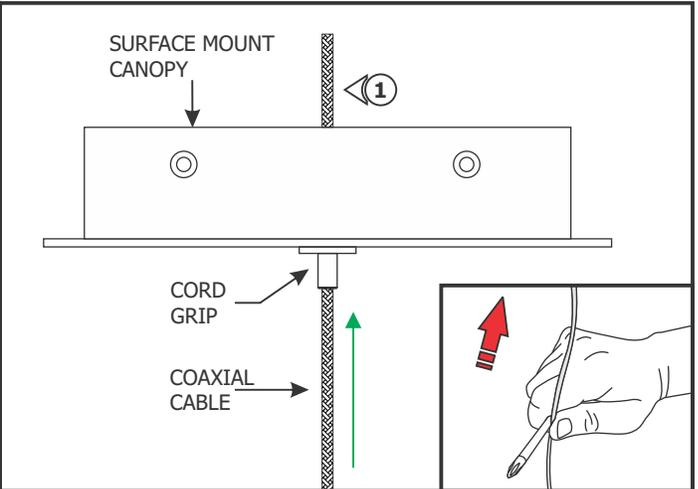
**NOTE:** If cable is curled or kinked, straighten by holding between the shaft of a screwdriver and thumb and pulling the cable through (see inset).
