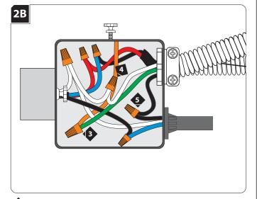
3 Ground the assembly properly in accordance with local electrical codes.
