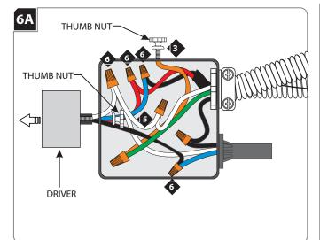
**CAUTION:**To reduce the risk of a burn or electric shock during the driver replacement, disconnect the power to the fixture.
