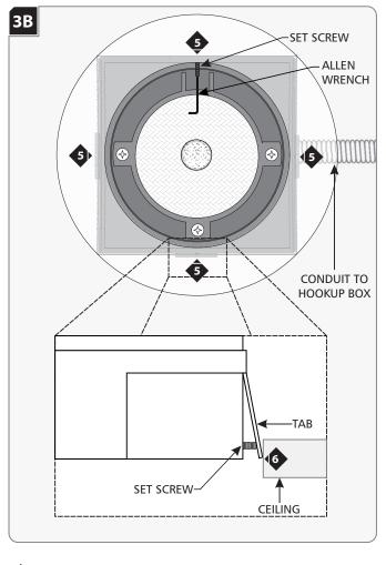
5 Secure the housing by screwing in the four set screws until they are flush with the inner wall of the housing. Alternate screws before tightening all the way to ensure housing remains centered in the ceiling cutout.
