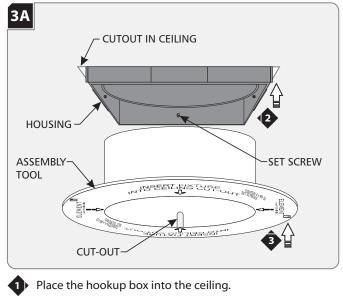
2 Slide the housing into the cutout in the ceiling.
