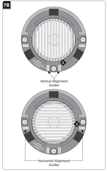
Use the lens orientation guides to align linear spread lenses vertically or horizontally.
