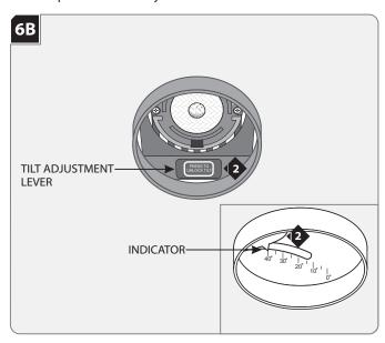
**NOTE:** Lamp housing can tilt 40° vertically. Lock intervals are 2.5° apart.
