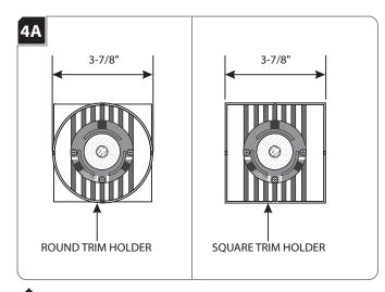
**1** For round trims, mark a 3-7/8" diameter circle on drywall. Cut out the marked section.
