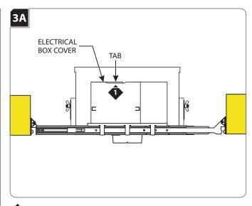
1 Push the tab on the housing electrical box up and remove the electrical box cover.
