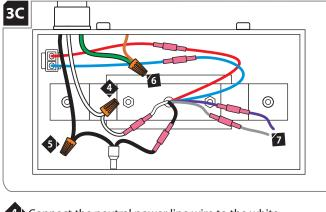
Connect the neutral power line wire to the white transformer wire with a wire nut.
