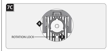
**NOTE:** Lamp housing can rotate 361° horizontally.
