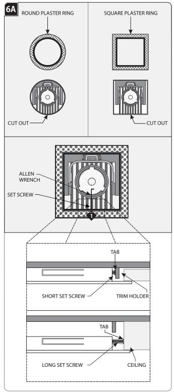
Insert the plaster ring completely into the collar/ceiling and secure them in place with the provided set screws and Allen wrench.
