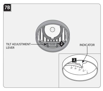
For proper wall wash positioning, unlock the tilt adjustment lever by pressing where indicated using a finger or screwdriver to tilt until 15° angle is reached.
