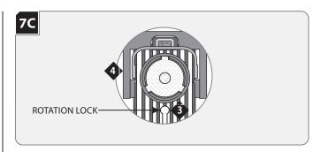
**NOTE:** Lamp housing can rotate 361°
