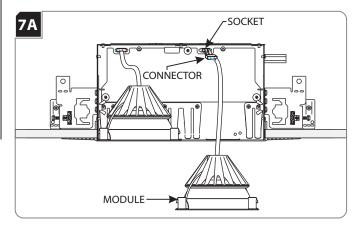
Push the module connector(s) into the electrical box socket(s) located inside the fixture housing.
