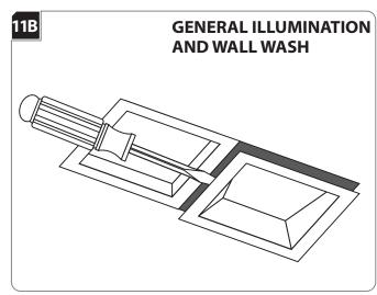
Remove the General Illumination and Wall Wash modules using a flathead screw driver to gently pry the module from the housing.
