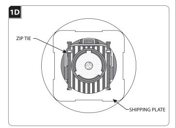
Carefully cut and remove the zip ties to remove the shipping plate.
