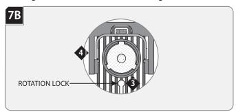
**NOTE:** Lamp housing can rotate 361° horizontally.
