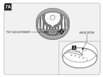
For proper wall wash positioning, unlock the tilt adjustment lever by pressing where indicated using a finger or screwdriver to tilt until 15° angle is reached.
