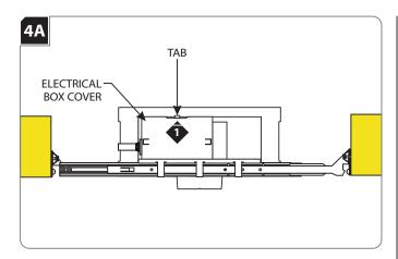
Push up on the tab on the electrical box and remove the electrical box cover.
