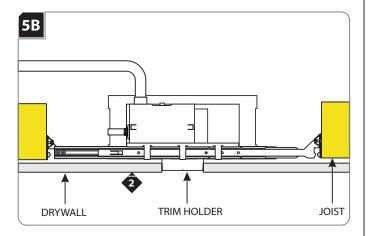
Align the cut out section of drywall with the trim holder and install the drywall.
