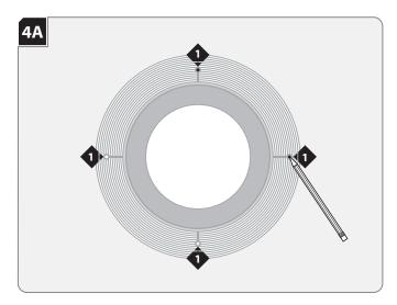
With the trim strain relief cable facing the location of the electrical box, hold the trim to the ceiling and mark the location of the mounting holes (4 holes for 5" and 8" sizes, 6 holes for 12" size).
