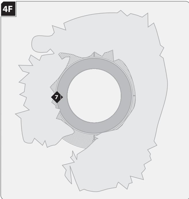
7 Properly plaster onto the plaster ring and drywall.
