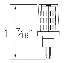
The 12V T5 EmeryAllen retrofit lamp is an energy efficient alternative to 12V incandescent T5 base lamps. It offers similar light output to a 12V, 20W incandescent (250lm) and is suitable for use in most 12V T5 base fixtures.
