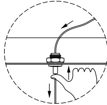
Stretching cable: Please hold down the bottom of the wire lock and slowly push or pull the cable down.
