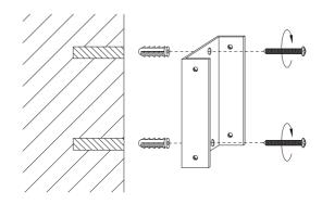
Set up the wall mount with two wall screws and two rawplugs.
