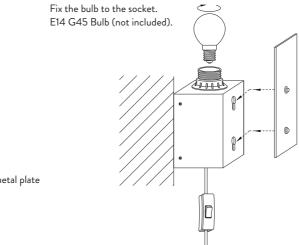
Fix the two hooks of metal plate into the key holes.
