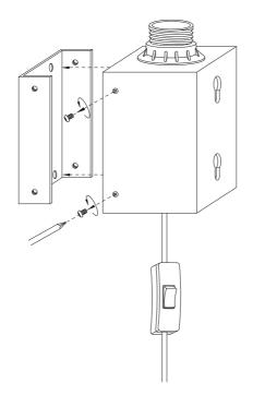
Unscrew the 4 wall screws on and remove the wall mount
