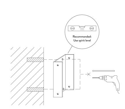
Use the wall mount to mark the two holes with a pencil. Drill two holes in the wall with a Ø5 drill
