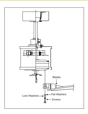
Fasten blade to motor with provided screws, lock washers and flat washers. Repeat procedure for remaining blades. Make sure screws are TIGHT! Loose motor screws can contribute to unnecessary hum during operation.
