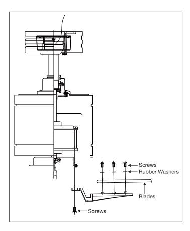
Place rubber washer on screw. Insert this assembly through the blade and start the screw into the blade arm. Repeat this procedure without tightening the screw until all 3 screws have been started into the blade arm.
