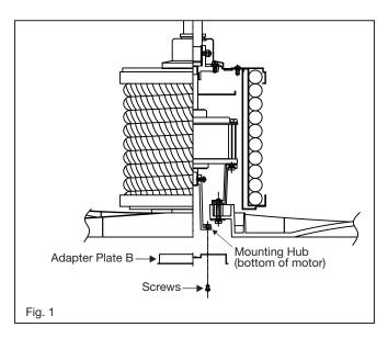
Remove one of the three screws on the mounting hub located on the fan motor. Loosen the other 2 screws. (Do not remove) (Fig. 1)
