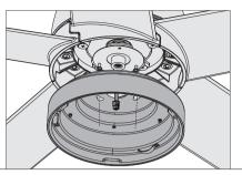
Feed the wire plug through the center hole of the uppers switch housing. Align the keyhole slots in the upper switch housing with the two screws you just installed. Lift the upper switch housing so that the keyhole slots engage the two screws, and twist counterclockwise to lock the upper switch housing into place.
