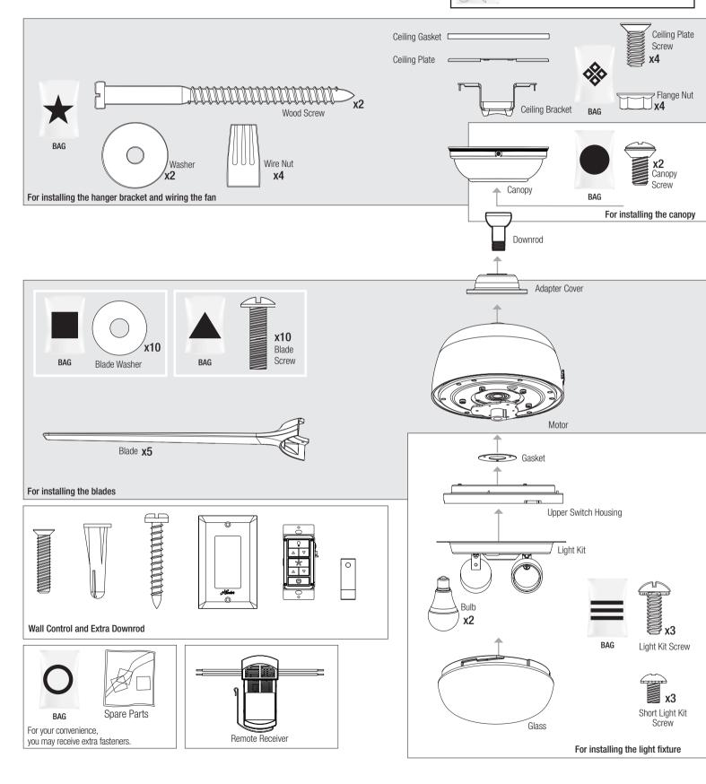
Note: Fan style may vary. Find a part that is missing or damaged?
