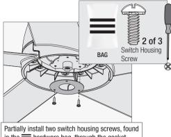
in the in the the ardware bag, through the gasket halfway into the motor housing as shown. It does not matter which two screw holes you choose.
