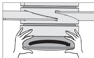
Attach the globe by lifting and turning clockwise one third of a full turn of the glass until it stops.
