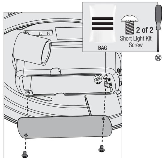
Carefully push all switch housing components into the switch housing, then install the switch housing plate using two short light kit assembly screws, found in the hardware bag.
