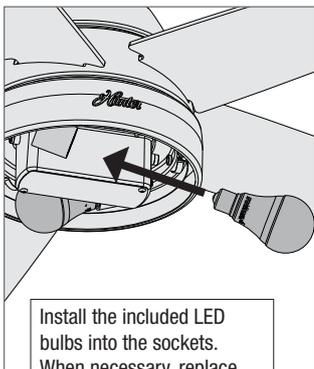
Install the included LED bulbs into the sockets. When necessary, replace with bulbs of same wattage.
