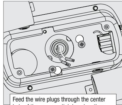
Feed the wire plugs through the center hole of the upper switch housing, then wrap keyhole slots around the screws and twist counterclockwise.
