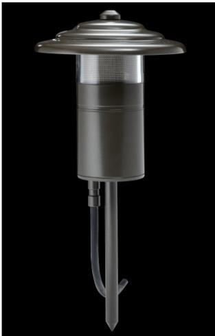
The Fern Lite is suitable for illumination of low level foliage. Light is emitted on a horizontal plane through UV stable acrylic lens with anti-glare mesh around 360 degrees. The luminaire uses a 5, 10 or 20 watt halogen bi-pin lamp and does not project any vertical light due to the anti-glare hood. The Fern Lite with no hood projects very little light due to the lens cap.
