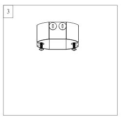
Use metal outlet box suitable for fan support and use only the screws provided with the outlet box (must support 35 lbs). Before attaching fan to outlet box, ensure the outlet box is securely fastened by at least two points to a structural ceiling member ( a loose box will cause the fan to wobble).
