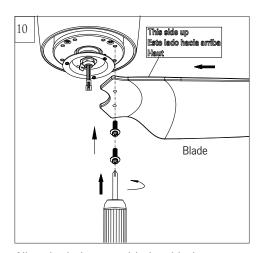
Align the holes on a blade with the screw holes on the motor, Install the blade using set screws provided. Repeat this process for other blades. Tighten all screws securely.
