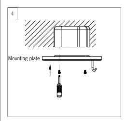
Remove the two screws provided with the outlet box, aligning the holes of the mounting plate with the screw holes of the outlet box. Reinstall the 2 outlet box screws securely.
