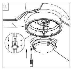
Connect light lead wires from fan to the lead wires from LED light fixture with quick connectors. Make sure the quick connectors are firmly clasped.
