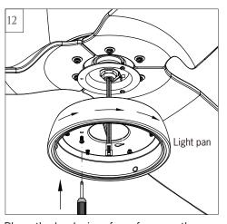
Place the lead wires from fan over the central hole of light pan
