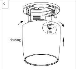
Attahced the housing onto the mounting plate. Align the tabs in the housing with the key hole slots on mounting plate as shown in the illustration and turn it clockkwise till tight.
