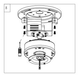
Attach motor assembly onto mounting plate.
