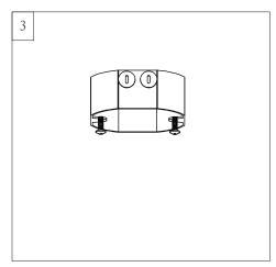
Use metal outlet box suitable for fan support and use only the screws provided with the outlet box (must support 35 lbs). Before attaching fan to outlet box, ensure the outlet box is securely fastened by at least two points to a structural ceiling member ( a loose box will cause the fan to wobble).
