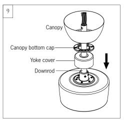
Place yoke cover, canopy bottom cap and canopy over lead wires, safety cable and downrod.
