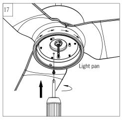
Place light pan over the lead wires and attach it onto the plate on motor, aligning the keyhole slots on the light pan with the preassembled screws on the plate. Twist clockwise till lock. Reinstall the set screws. Tighten all the set screws securely.
