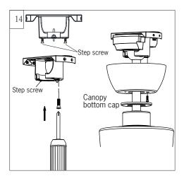
Partially loosen one and remove one preassembled step screw from mounting bracket (Do not remove the other set screws). Save the screw.
