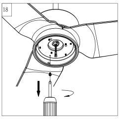
Loosen 2 and remove 1 preassembled screw from the light pan. Save the screw for later use.
