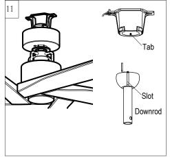
Install ball end of downrod into mounting bracket opening. Align (engage) slot on ball with tab on mounting bracket.
