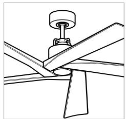
Lift canopy up, aligning its keyhole slot with the preassembled screw on mounting bracket and twist counterclockwise to lock in place. Reinstall the screw removed in step 14 and tighten all screws securely. Attach canopy bottom cap onto canopy by aligning its notch with the screws on mounting bracket and twist clockwise till tight.
