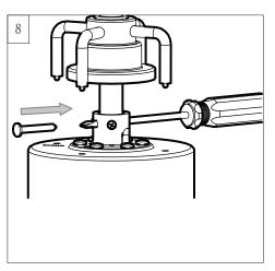
Helpful hint: For easy assembling of the cross pin on the next installation step.
