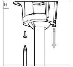
Partially loosen one and remove one preassembled screw from mounting bracket. Save screw.
