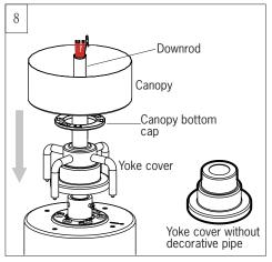
Place yoke cover, canopy bottom cap and canopy over the downrod. An optional yoke cover without decorative pipe provided.
