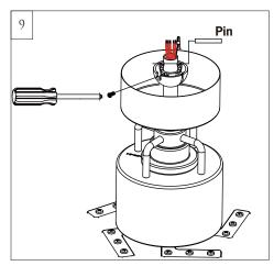
Replace the hanger ball with pin and set screw. Tighten it securely. **Warning**: Make sure the **pin** is installed well on hanger ball with downrod.
