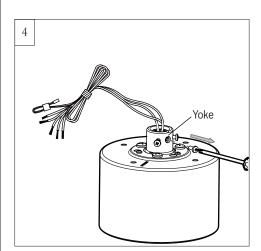
Remove downrod set screws from the yoke on top of motor assembly. Keep the screws.
