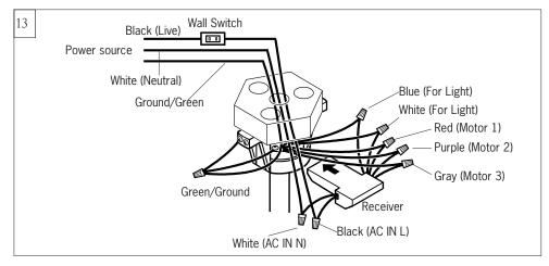
Make wiring connections using wire connectors provided as indicated above.
