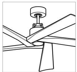
Lift canopy up, aligning its keyhole slot with the preassembled screw on mounting bracket and twist counterclockwise to lock in place.
