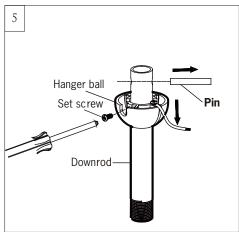
Remove hanger ball from downrod by loosing the set screw and removing the pin as shown in illustration. Keep parts.
