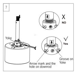
Spin the downrod into the yoke on top of fan until the hole with the arrow mark on downrod is close and aligned with the gloove on top edge of the yoke, and then reinstall the screws securely.
