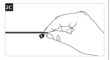
4 Cut the coaxial cable to the desired length.
