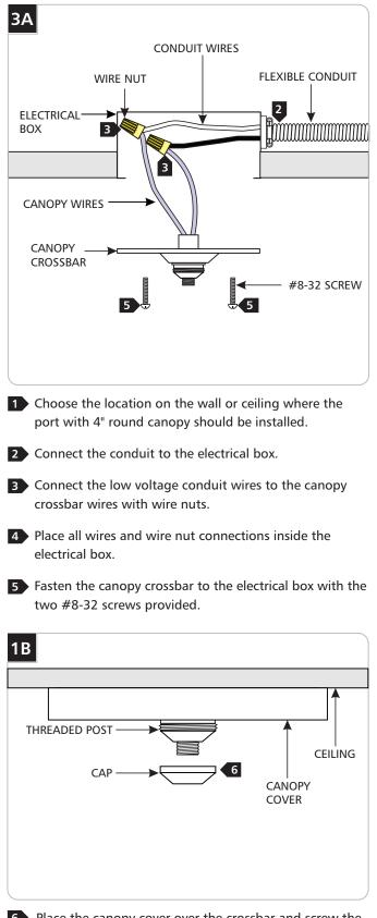
6 Place the canopy cover over the crossbar and screw the cap onto the threaded crossbar post.
