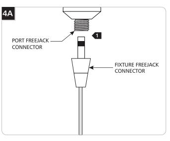
1 Tighten the fixture FreeJack connector completely into the port FreeJack connector.
