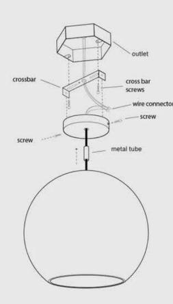
4/ Connect White house wire from outlet box to White wire from fixture using wire connector. Connect Black house wire from outlet box to Black wire from fixture using wire connector.
