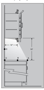
**Over Cabinets** Trac 12, using TL103LEDs spaced 12" on-center, generally provides excellent indirect lighting. For lower-level mood lighting, use TL103LEDs with closer lamp spacing. Placing the fixture at the front edge of the cabinet top will project light into the space and illuminate any displayed objects. Locate top of lamp even with top edge of cove molding to prevent a harsh shadow line.
