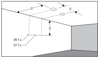
EXAMPLE: With multiple clear reflector units located 3' from wall and spaced 3' on center, the illumination on the wall 3' down from ceiling will be 36 f.c. beneath units and 37 f.c. between units.
