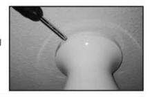
(6) Remove and set aside bottom cap by rotating counter-clockwise.
