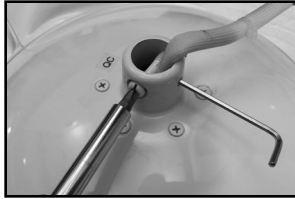
Remove stopper screw & loosen hex screw
