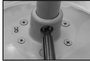
Reinstall stopper screw
