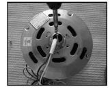
(3) Using screws from step (2), attach the canopy to fan body.
