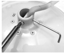
remove stopper screw and loosen hex screw
