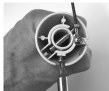
remove half-ball and stopper pin
