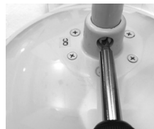
reinstall and tighten stopper screw
