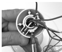
reinstall half-ball, stopper pin and tighten set screw
