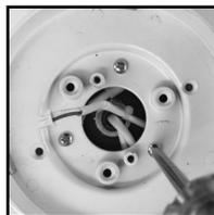
Place light cup over wire connectors so that the three posts are seated in holes on back of light cup and two pin connector passes through center hole. Use three countersink screws to fasten light cup in place.
