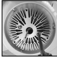
Route bridge connector through center of heatsink and place heatsink inside light cup so that fastening holes are aligned over two fastening posts. Using the long panhead screws, secure heatsink in place with screw heads recessed into milled side of heatsink.
