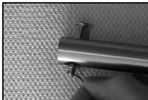
Remove stopper pin, cottor pin and washer
