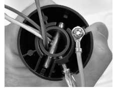
reinstall half-ball with stopper pin and tighten set screw
