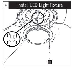
Connect white wire from fan to white wire from LED light fixture and then connect blue (or black) wire from fan to black (or blue) wire from LED light fixture. Be sure plugs connection clasped together firmly. Attach LED light fixture onto the light pan, aligning the keyhole slots on the LED light fixture with the preassembled screws on the light pan. Twist clockwise till lock. Reinstall the screw which was just removed. Tighten all screws securely.
