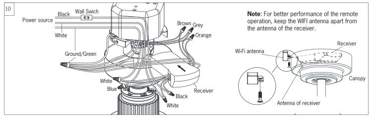
Make wiring connections using wire connectors provided as indicated above. Brown wire from fan to Brown wire from receiver marked Motor U. Gray wire from fan to Gray wire from receiver marked Motor V. Orange wire from fan to Orange wire from receiver marked Motor W. White wire from fan marked "For light" to White wire from receiver marked "For light". Blue wire from fan marked "For light" to Blue wire from receiver marked "For light".
