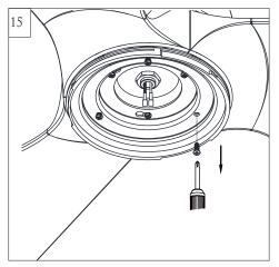
Loosen 2 and remove 1 preassembled screws from light pan. Keep screw.
