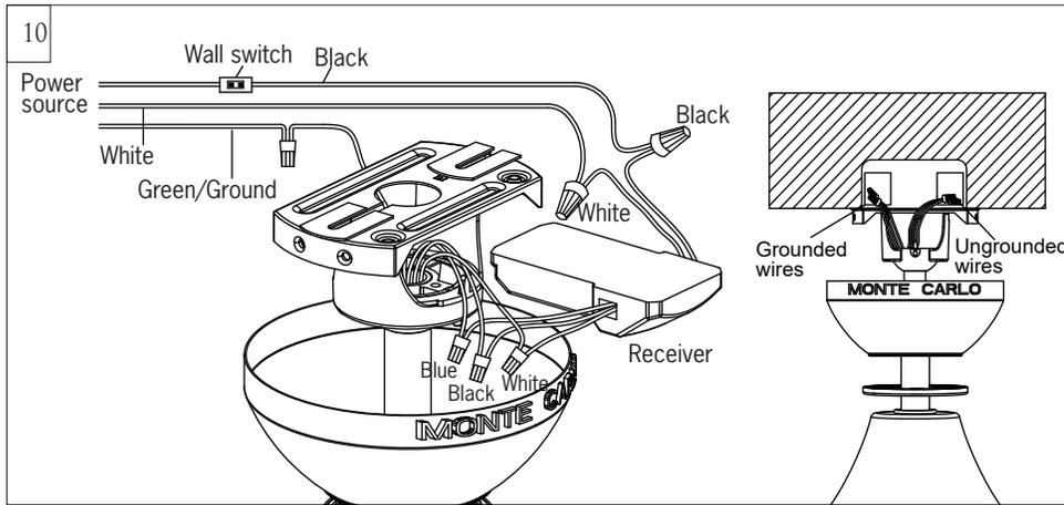
Make wiring connections using wire connectors provided as indicated above. White from fan to White from remote marked to motor N. Black from fan to Black from remote marked to motor L. Blue from fan to Blue from remote marked FOR LIGHT. White (Neutral) from house to White from remote marked AC IN N. Black (Live) from house to Black from remote marked AC IN L. Connect all green grounded wires to Grounded wire from House. Make sure that no filaments are outside of the wire connectors.
