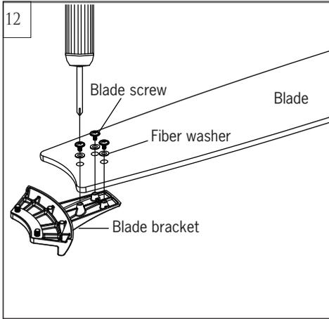
Install blade bracket with blade by using blade set screws and fiber washers provided. Tighten screws securely. Repeat this process for remaining blades.
