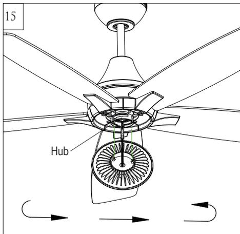
Install the LED light fixture onto the hub on the fan. Place light lead wires in the hub and attach LED light fixture onto the hub by locating ridges in the LED light fixture with the grooves on the hub and twist clockwise until tight. **Caution:** Make sure the lead wires are placed in the hub and keep them from damage.
