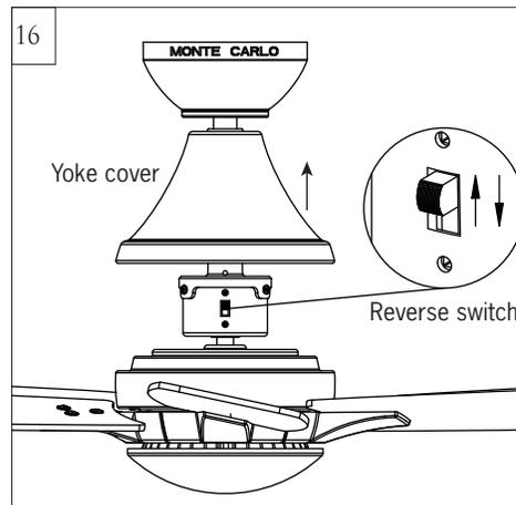
Setting the reverse switch in the down position will result in downward airflow and setting the switch in the up position will result in upward airflow. **Note:** Reverse switch must be set either completely down or completely up for fan to function. If the reverse switch is set in the middle position, fan will not operate.
