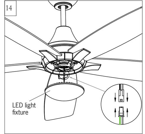
Connect the light lead wires from fan to LED light fixture with a quick connector as shown in the illustration. **Note:** Be sure quick connector clasped together completely.
