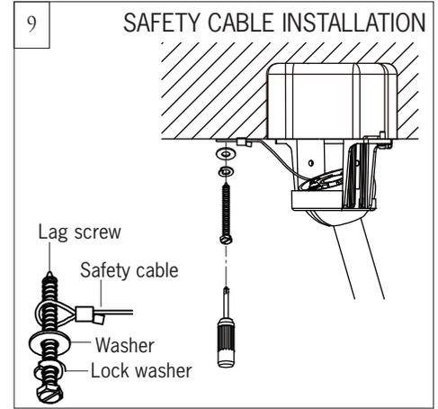
For Canadian installation and for USA fan and light kit combinations over 35 lbs, in both flush and downrod modes the safety cable must be installed into the house structure beams using 3" lag screws, washers and lock washers provided.
