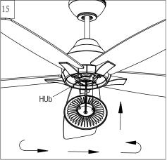
Install the LED light fixture onto the hub on the fan.
