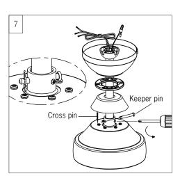
Slip downrod into motor housing voke. aligning holes and install cross pin and keeper pin.
