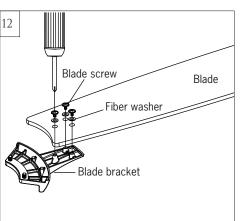
Install blade bracket with blade by using blade set screws and fiber washers provided. Tighten screws securely. Repeat this process for remaining blades.
