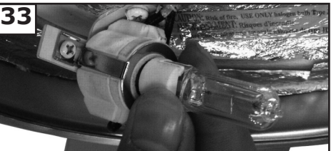
33 Install a JD 75 watt halogen bulb, bulb included. Caution: Do not replace bulb until it cools down. WARNING: Over lamping the fan will result in the fan lights shutting down until the proper wattage of bulbs are installed. Reset the lights by turning off the wall switch, breaker, or by remote. Replace bulbs with the correct wattage bulbs, turn the power on.
