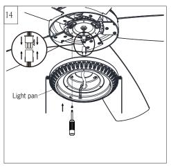
Connect the quick connector from fan to the quick connector from switch house (light pan). Be sure they are clasped together firmly.
