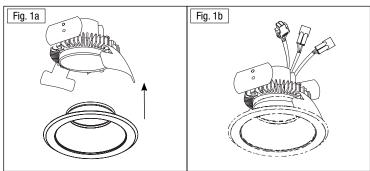
The NLCBC2-4 trims simply "Click" in place on the Cree LED engine allowing Nora, the end user or distributor to easily change from a standard trim to an application specific trim.
