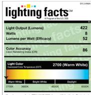
All results are according to IESNA LM-79-2008: Approved Method for the Electrical ar Photometric Testing of Solid-State Lighting. The U.S. Department of Energy (DOE) verificonduct test data and results.
