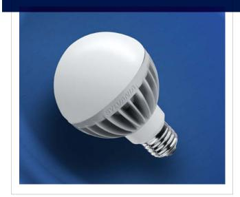
LED technology offers reduced energy and maintenance costs when compared with conventional light sources. Consuming only 8W and lasting 33 times longer, LED G25 retrofit lamps are high-quality replacements for 40W incandescent lamps. They are free of UV and IR radiation minimizing discoloration and fading of materials. These lamps are dimmable down to 10%\* and rated at 50,000 hours life with a correlated color temperature (CCT) of 2700K and 3000K.
