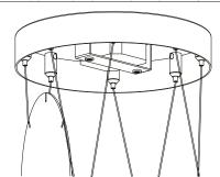
Thread screws into JUNCTION BOX or appropriate ceiling anchor. Use keyholes to place canopy onto the ceiling, rotate, then fasten mount screws as necessary.
