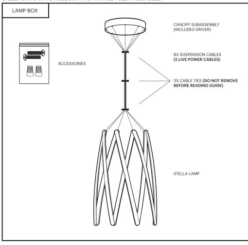
ITS CRITICAL TO AVOID TANGLING THE CABLES PRIOR TO INSTALLATION. PLEASE TAKE EXTRA CARE WHEN REMOVING THE LAMP FROM ITS PACKAGING TO KEEP THE ENTIRE ASSEMBLY IN ALIGNMENT.
