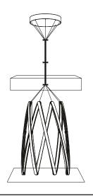
2 Remove Upper Most cable tie. Push on one end of the CANOPY COVER PLATE to release magnetic connection.
