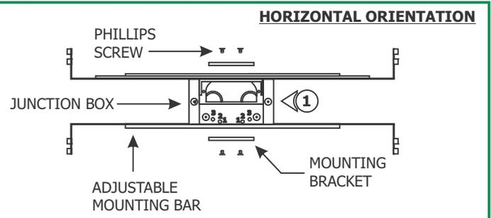
**1:** Determine channel orientation. Mount each adjustable mounting bar to one side of the junction box and secure them with the provided mounting brackets and two Phillips screws.
