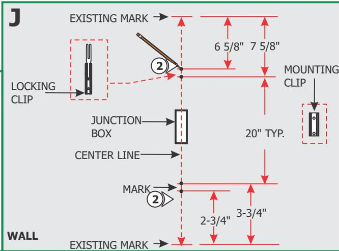
**NOTE:** Steps 3 and 4 are for drywall mounting. Omit these steps if mounting the clips to a wood surface directly.
