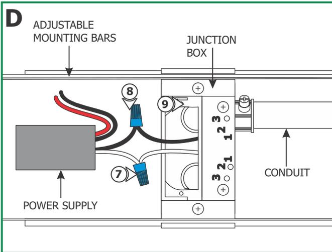
**NOTE:** Make sure that the junction box is at position 3 (1.05") so that the power supply fits easily.
