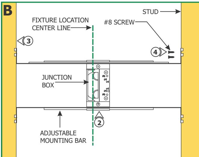
**NOTE:** The adjustable mounting bars mount to studs that are spaced 13" to 24" apart.
