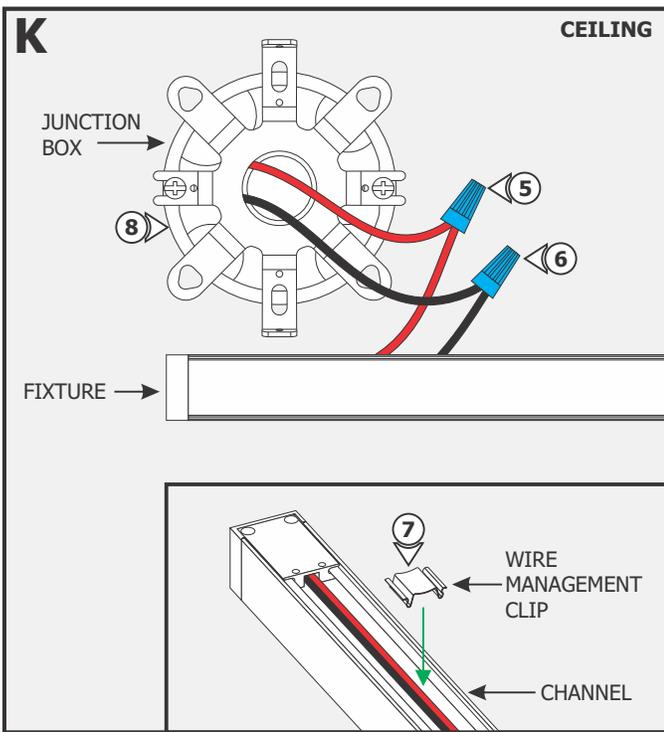
**5:** Connect the low voltage +24VDC power supply wire to the red wire of the fixture with a wire nut.
