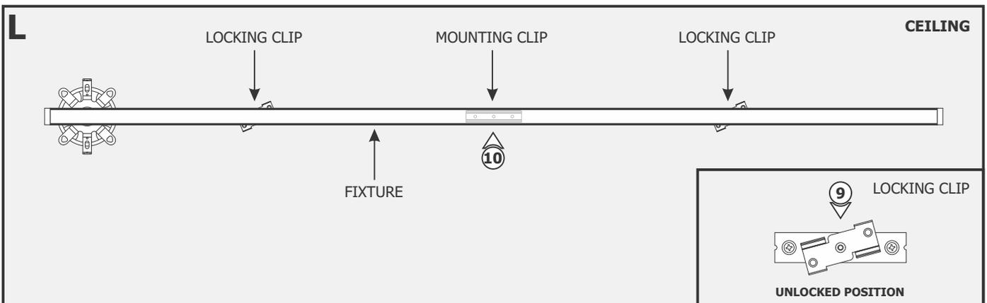
**9:** Make sure the locking clips are in the unlocked position before installing the fixture to the mounting clips.
