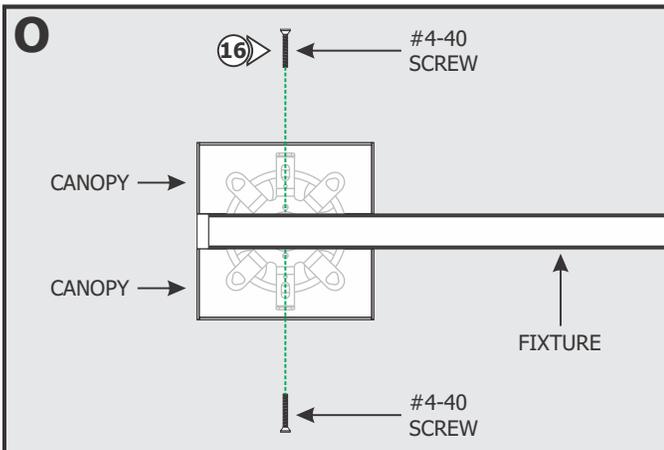
**16:** For 4" Square Split Canopy installations, place each canopy piece against the fixture and align the canopy holes with the crossbar holes. Secure the canopy pieces in place with the two #4-40 screws and 1/16" Allen wrench provided.
