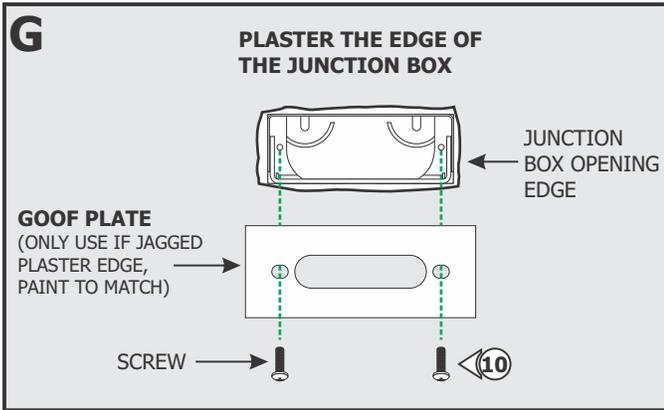
**10: Optional:** Use the Goof Plate if the junction box opening has imperfection/ jagged edges. Install the provided goof plate (paint to match prior) with the two screws.
