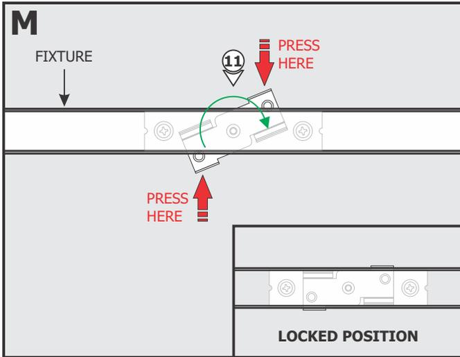
**11:** Twist each locking clip to lock the fixture in place.
