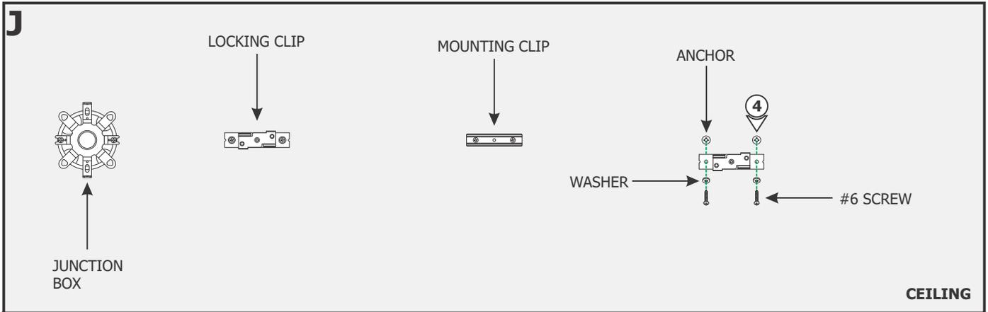
**4:** Line up the locking clips and mounting clips to the anchors and secure them by tightening the two #6 screws through the washers and clip holes into the anchors.
