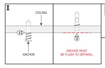
**NOTE:** Steps 2 through 4 are for drywall mounting. Omit these steps if mounting the clips to a wood surface directly.
