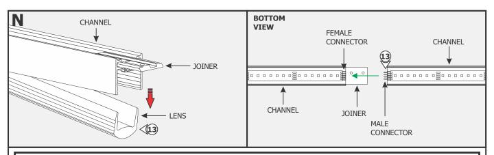
NOTE: Omit steps 12 through 15 if the channel is made out of a single piece (120" or less).
