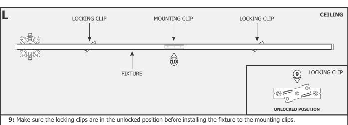
10: Carefully SNAP the channel onto the mounting clips. Make sure not to nick the wires.
