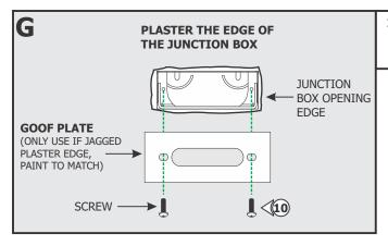
**10: Optional:** Use the Goof Plate if the junction box opening has imperfection/ jagged edges. Install the provided goof plate (paint to match prior) with the two screws.
