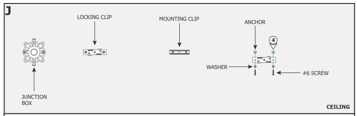
**4:** Line up the locking clips and mounting clips to the anchors and secure them by tightening the two #6 screws through the washers and clip holes into the anchors.
