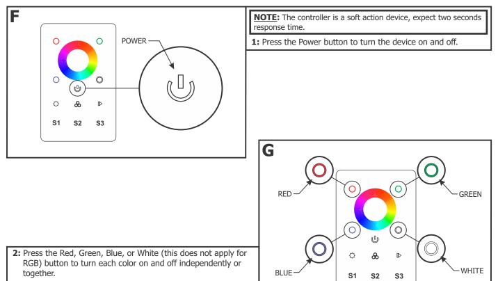
**3:** To adjust the brightness of each color, press and hold the color button.
