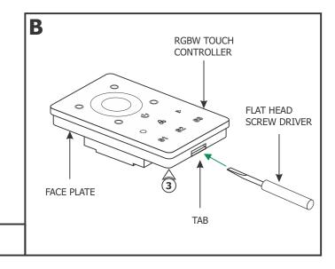
**3:** Pry the face plate of the RGBW Touch Controller using a flat head screw driver.
